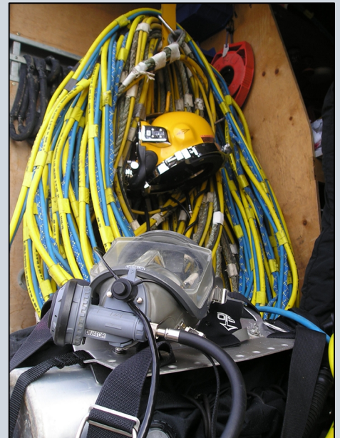
Surface supplied helmet and band mask with hardwire communications
